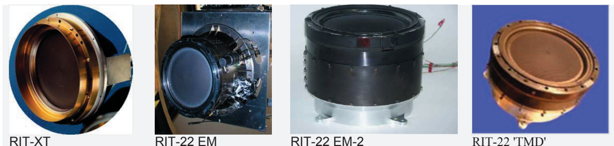
Figure 3 Evolution of the RIT-22 High Power Ion Thruster
